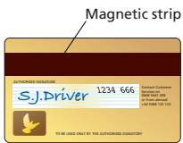
Figure 2.2 The magnetic stripe on a credit card
